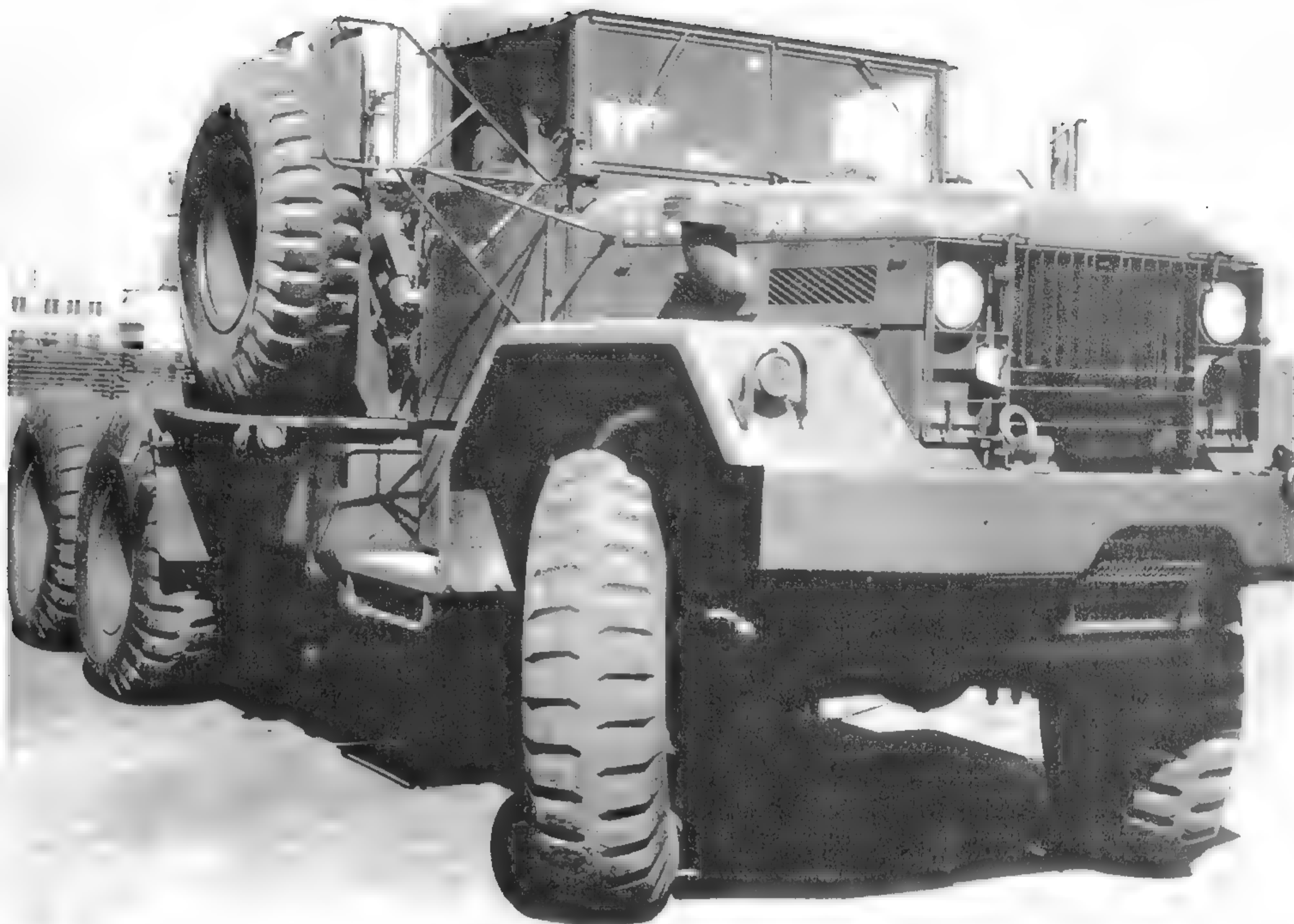
A quick distinguishing feature of the diesel-powered trucks is the intake air elbow on the passenger-side engine side panel. Notice the access step folded up neatly in the center of the bumper. (Photo courtesy of the Mack Trucks Historical Museum)
